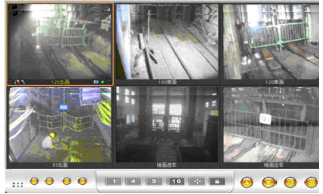
Fig. 11. The remote video surveillance for the coal mine, which can provide the first-hand image data for the analysis of accidents.
