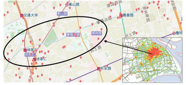
Fig. 3. An example of elliptic region based method on base stations from Shanghai Telecom Industry. A bubble in the picture means a base station deployment at its place. This is an enlarged image for a certain position of the map at the bottom right corner. And it is a heat map that shows the Shanghai overview of distribution density of base stations.
